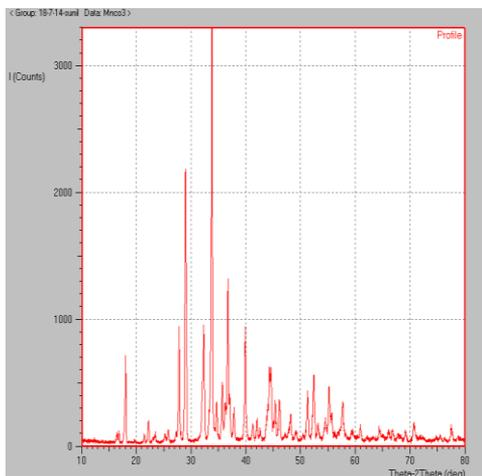
Figure.3: XRD of Manganese Carbonate.
