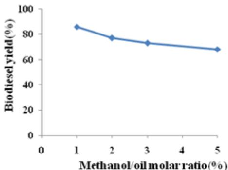
Fig.5. Effect of methanol/oil molar ratio
