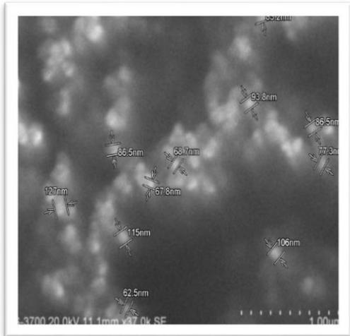
Figure 4: SEM Image of Manganese Carbonate
