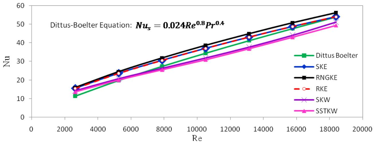
Fig. 2. Smooth duct analysis for selection of suitable turbulent model
