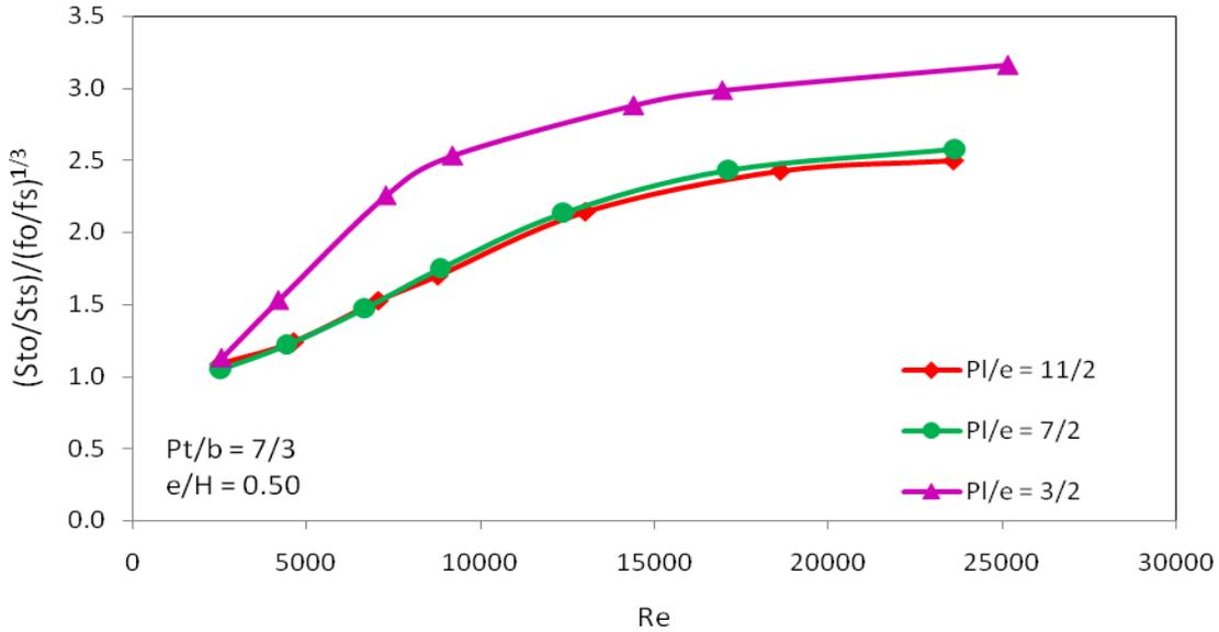
Fig. 15: Effect of relative obstacles longitudinal pitch ( $Pl/e$ ) on thermo-hydraulic performance  $\alpha = 60^\circ$ ,  $e/H = 0.50$  and  $P_t/b = 7/3$
