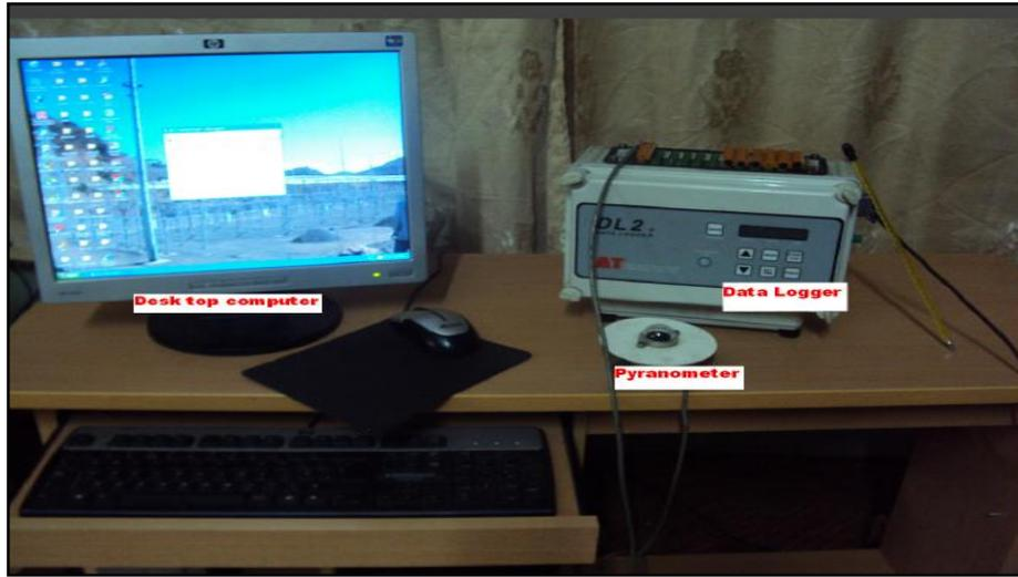
Figure 3: Pictorial representations of DL2e Data Logger and pyranometer
