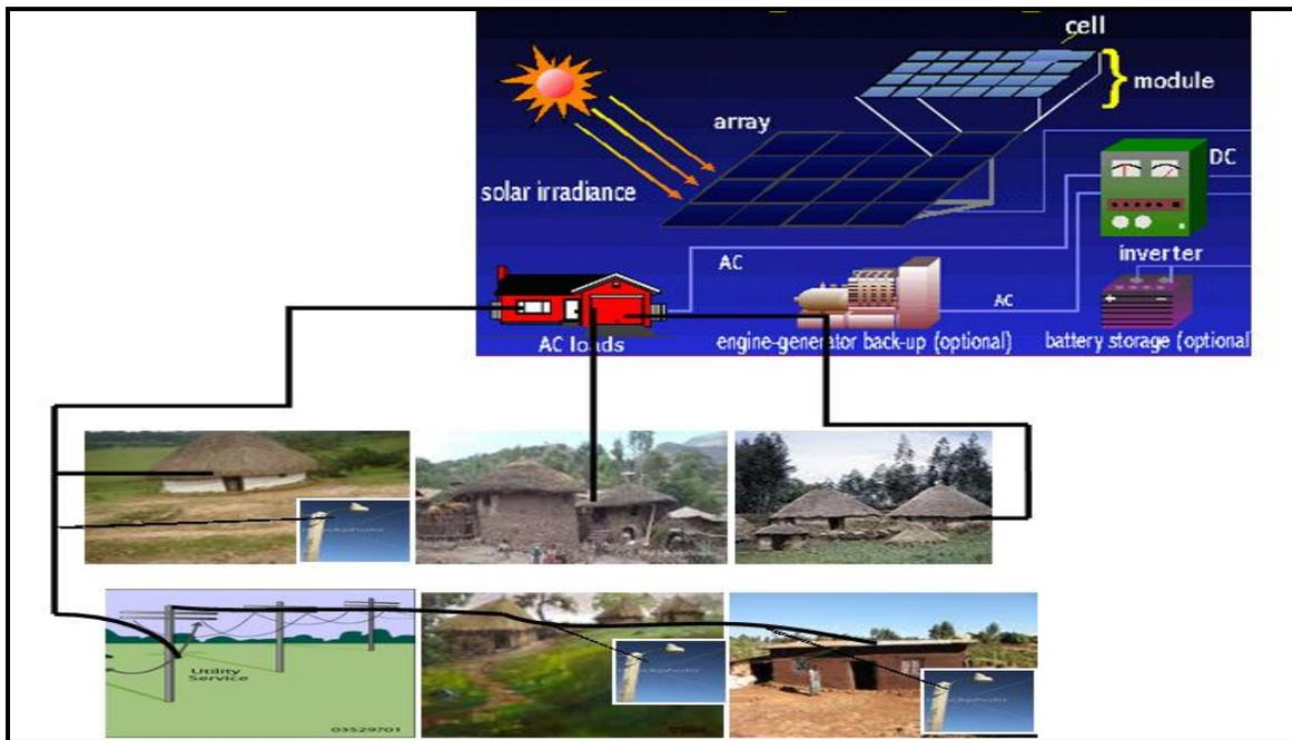
Figure 7: Schematic representation of single-phase line configuration of PV-diesel hybrid Power system
