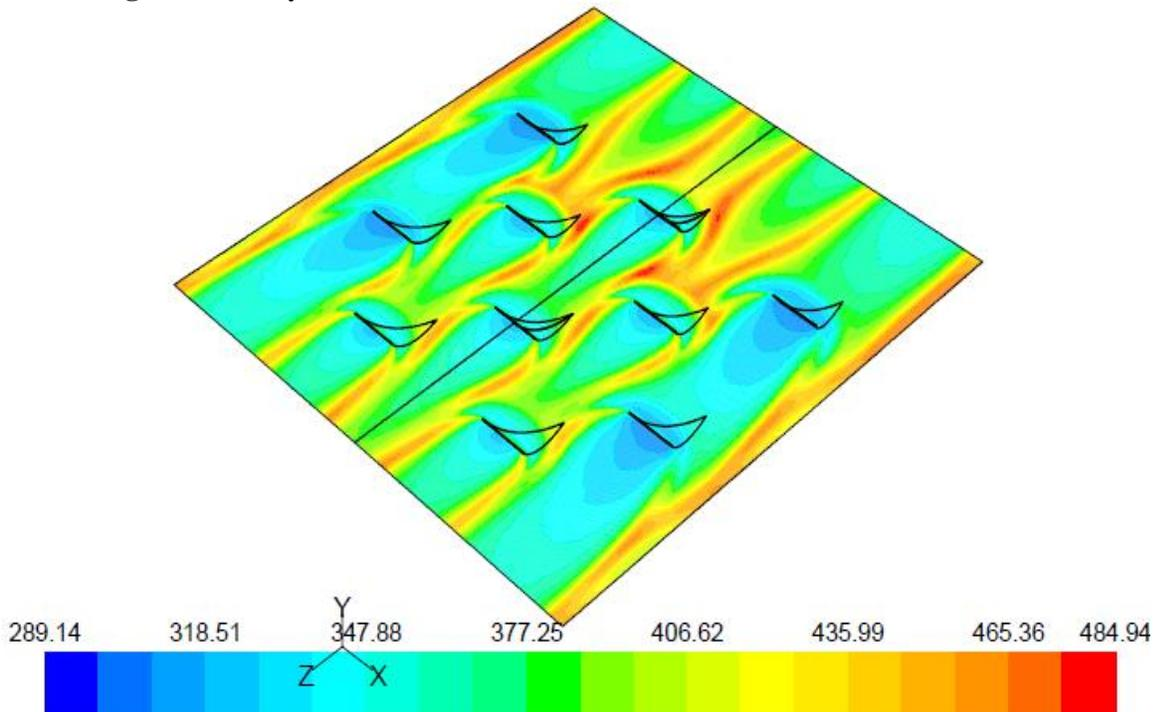
**Fig. 10.** Static temperature contours for  $P_v/e = 3/2$ ,  $P_v/b = 7/3$ ,  $e/H = 0.50$ ,  $\alpha = 60^\circ$ ,  $Re = 3000$
