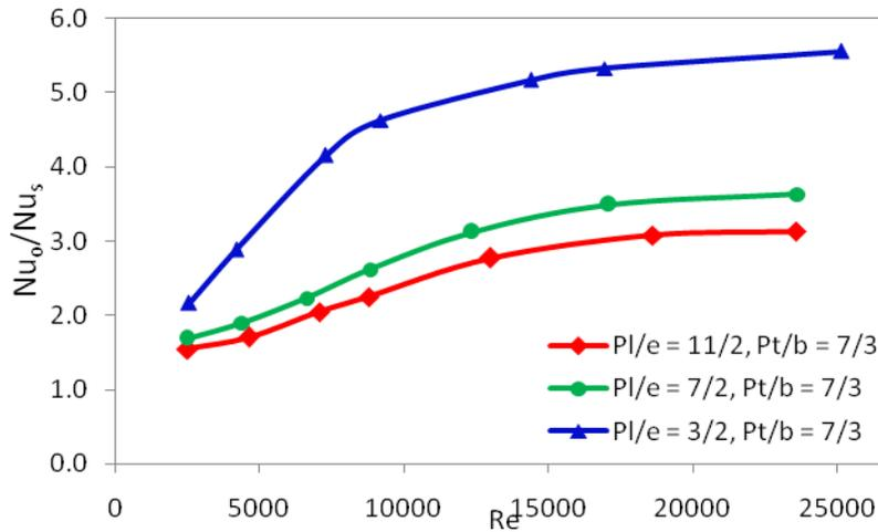
Fig. 13. Enhancement in Nusselt number ( $Nu_o/Nu_s$ ) as a function of Reynolds number ( $Re$ ) for  $e/H = 0.50$  and  $\alpha = 60^\circ$
