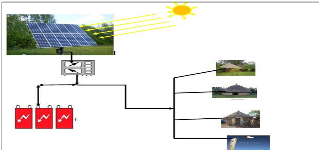
Figure 8: Schematic representation of PV installation for Gojo houses far from power house
