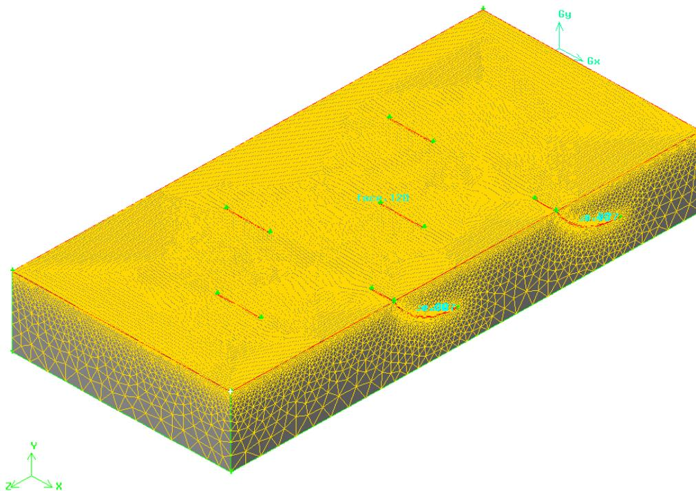
Fig. 4. Mesh of computational model  $P_l/e = 3/2$ ,  $P_f/b = 7/3$ ,  $e/H = 0.50$ ,  $\alpha = 60^\circ$ ,
