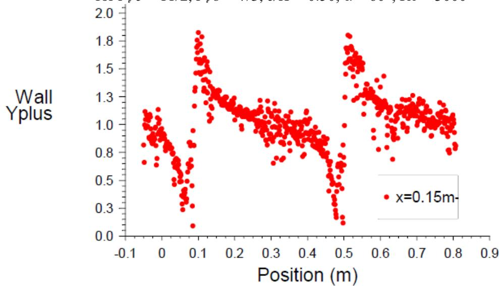
Fig. 7. Wall  $Y^+$  plot on the center line of absorber plate for  $P_l/e = 11/2$ ,  $P_l/b = 7/3$ ,  $e/H = 0.50$ ,  $\alpha = 60^\circ$ ,  $Re = 3000$
