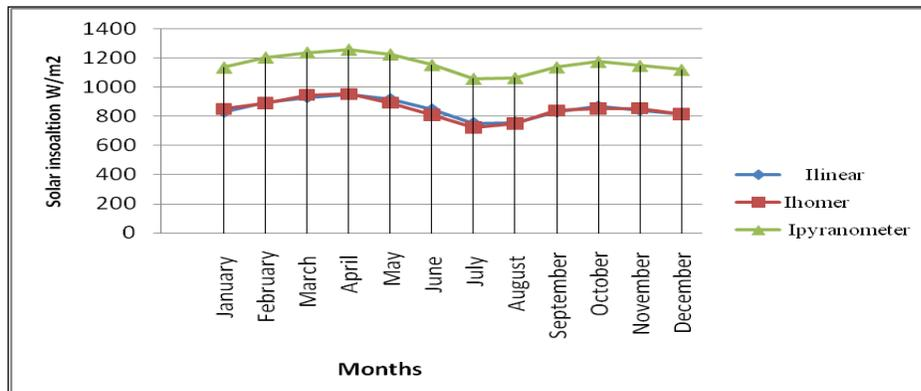
Figure 4: Daily average solar insolation results data using pyranometer, linear regression and homer.
