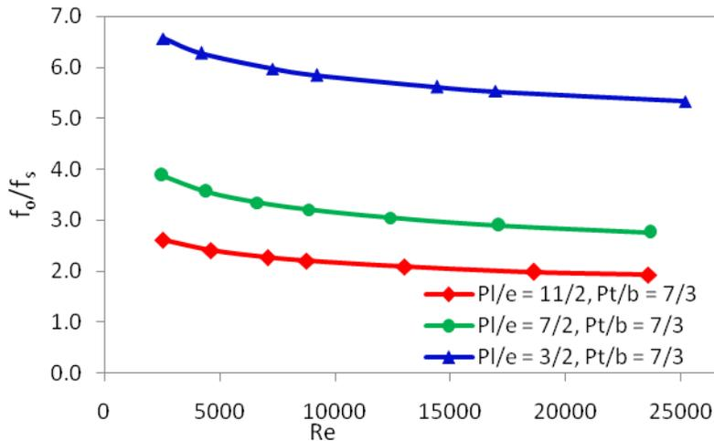
Fig.14: Enhancement in friction factor ( $f_o/f_s$ ) as a function of Reynolds number ( $Re$ ) for  $e/H = 0.50$  and  $\alpha = 60^\circ$
