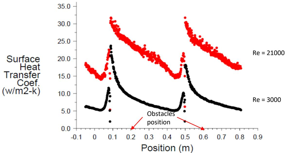
Fig. 12. Surface heat transfer coefficient along the obstacles for  $P_l/e = 11/2$ ,  $P_l/b = 7/3$ ,  $e/H = 0.50$ ,  $\alpha = 60^\circ$
