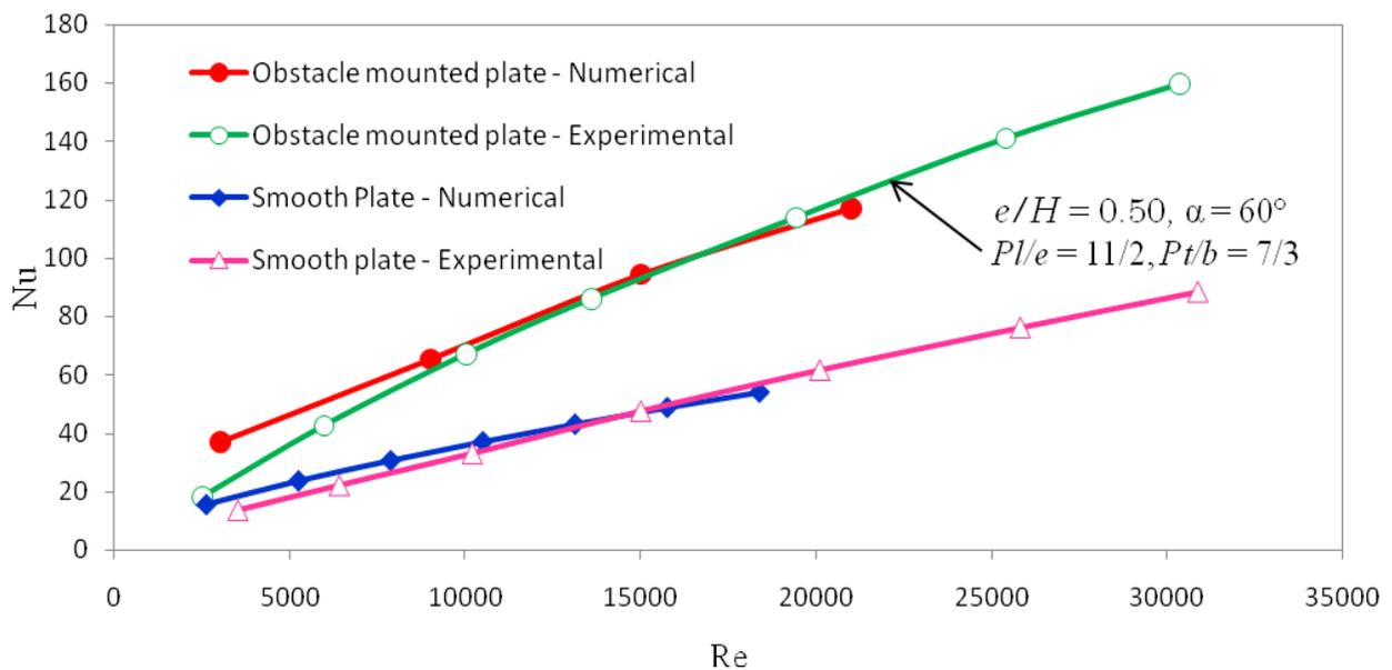
Fig. 3. Validation of the numerical result using the  $Rk-\epsilon$  model with the corresponding experimental Result
