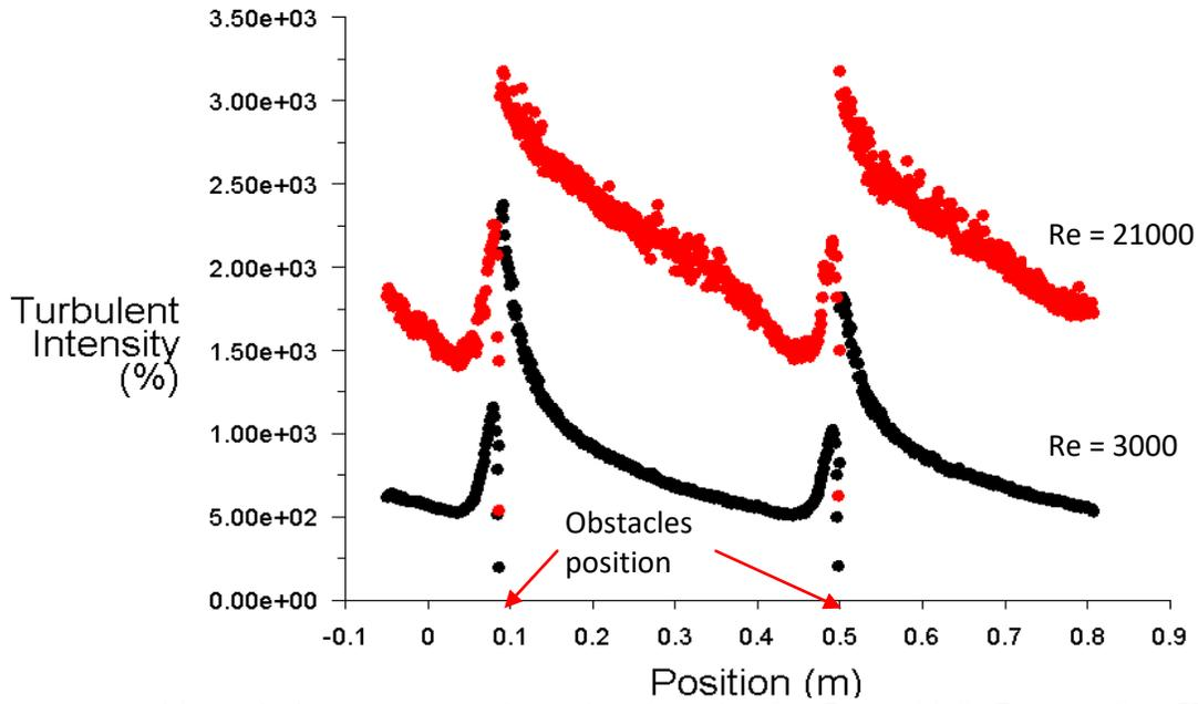
Fig. 11. Turbulent intensity along the obstacles for  $P_l/e = 11/2$ ,  $P_l/b = 7/3$ ,  $e/H = 0.50$ ,  $\alpha = 60^\circ$
