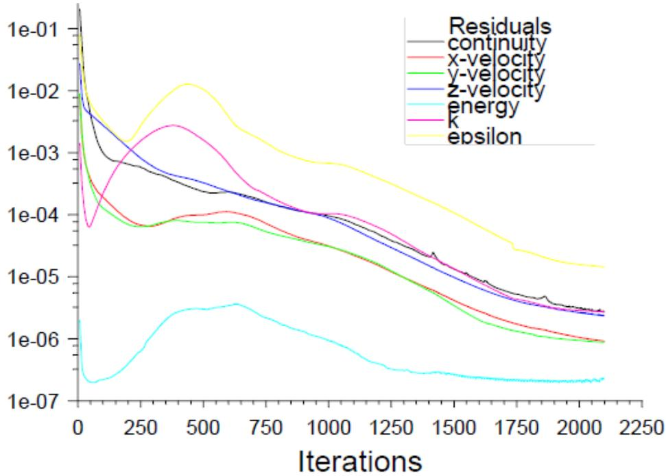
Fig. 5. Convergence plot of scaled residuals for  $P_l/e = 11/2$ ,  $P_l/b = 7/3$ ,  $e/H = 0.50$ ,  $\alpha = 60^\circ$ ,  $Re = 3000$
