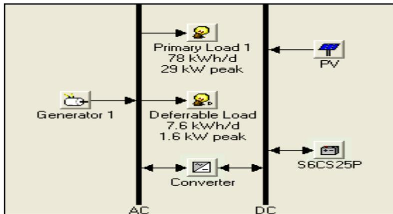
Figure 5: HOMER diagram for the hybrid PV-generator-battery-converter set up
