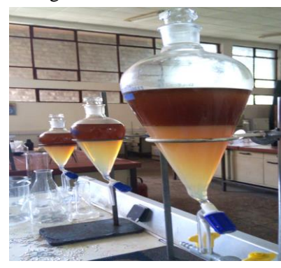
Figure 5: Washing biodiesel (soap is at bottom)
