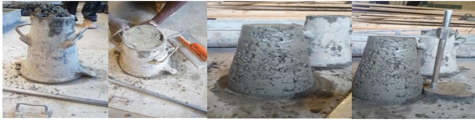
Figure 8: Property of fresh RRPC by slump test
