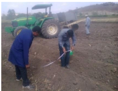
Figure 6: Checking the furrow spacing and depth created by the planter
