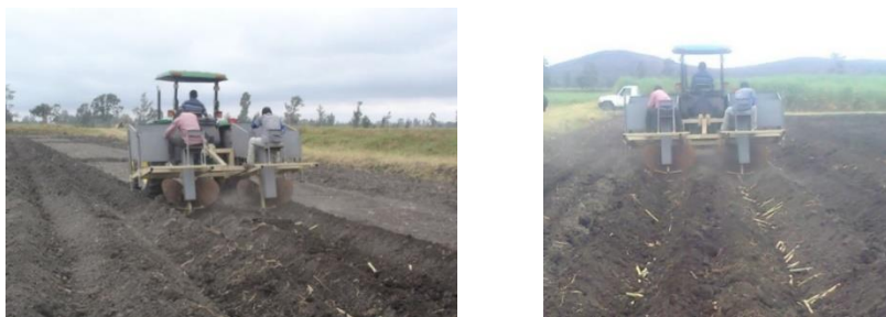
Figure 7: Planting cane with the developed planter
