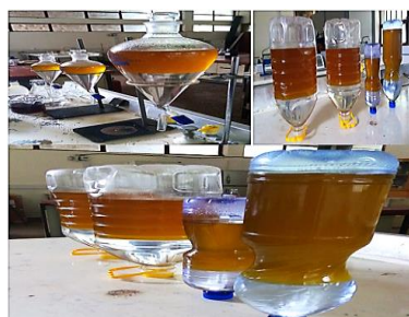
Figure 6: Final washing of biodiesel
