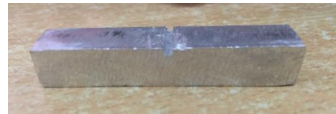
Figure 4: Charpy Impact Test Specimen as per ASTM-E-23
