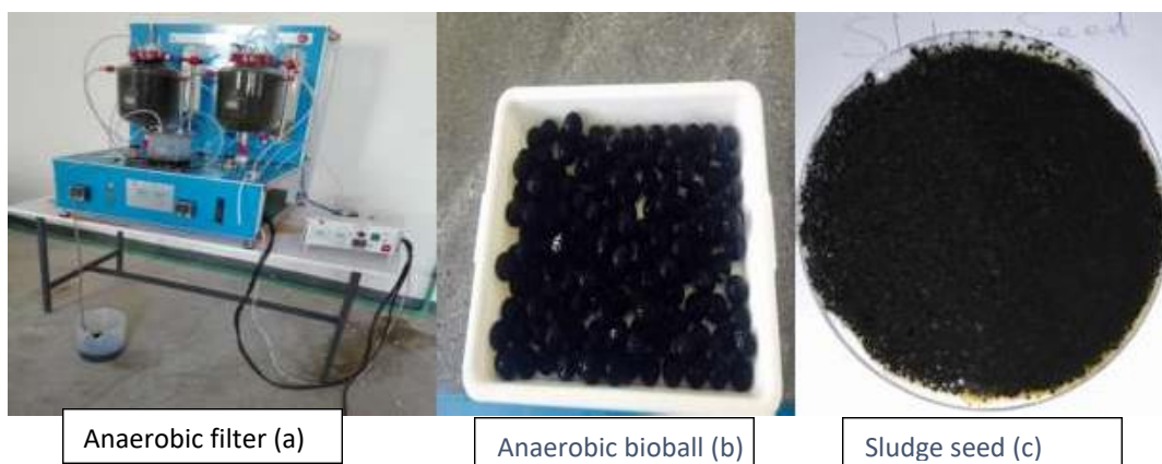
Figure 3: Two-stage water jacketed anaerobic filter (a), anaerobic bioball (b), and sludge seed (c) used in the bioreactor
