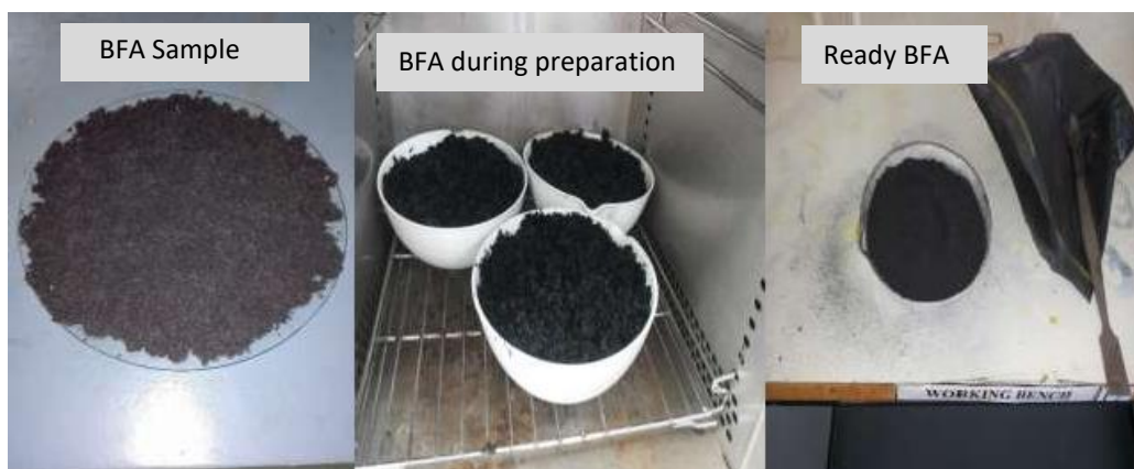
Figure 4: Adsorbent preparation stages of the BFA
