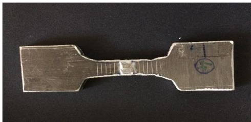
Figure 5: Tensile Testing Sample as Per ASTM-E8/E8M-09
