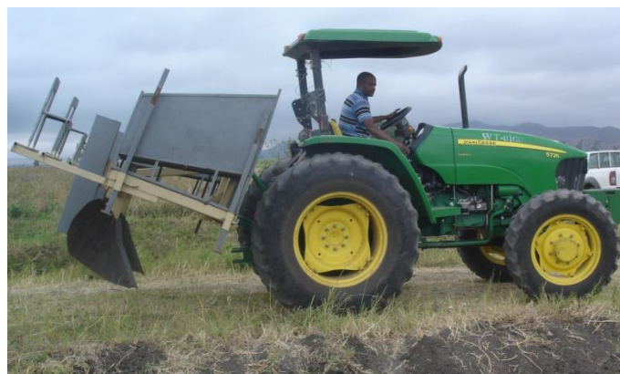
Figure 5: The completed planter ready for field testing
