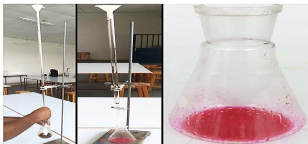
Figure 2: Titration to find FFA in the oil
