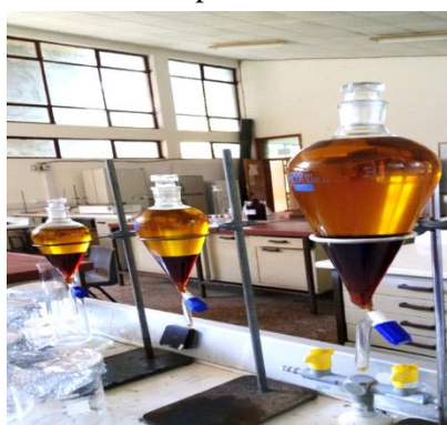
Figure 4: Glycerol Separation from methyl ester
