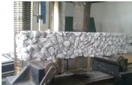
Figure 3.2: Flexural strength test
