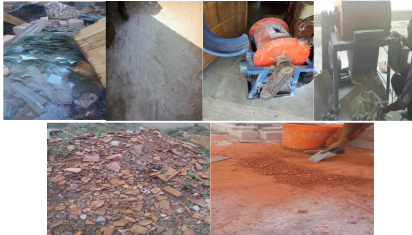
Figure 3: Preparation of Waste glass, waste ceramic, waste brick.
