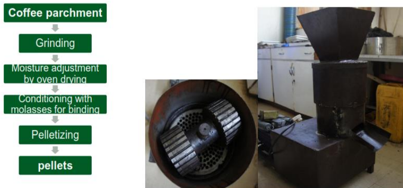
Figure 2: pellet formation phases from coffee parchment and pelletizing machine used
