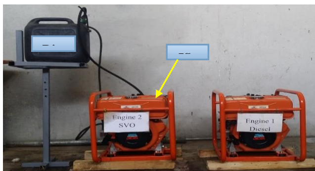
Figure 3: Overall picture of experimental setup for dual fueling and diesel engine
