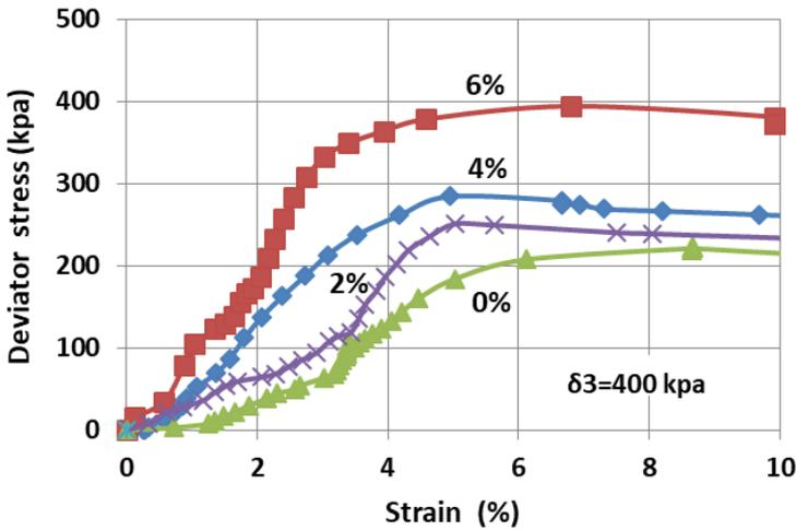
Figure 5. Influence of different lime content on the compressive strength of soil (TP-1)
