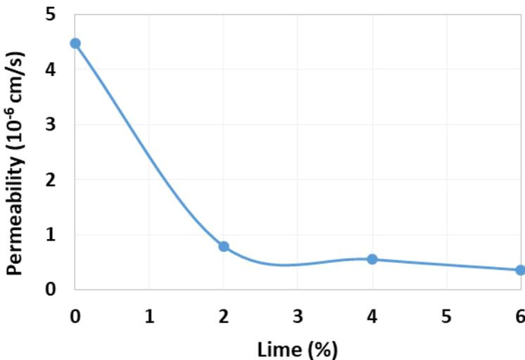
Figure 6. Influence of lime content on the hydraulic conductivity of soil (TP-1)
