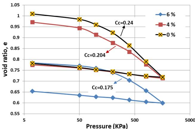
Figure 4. Influence of lime on the compressibility characteristics of soil (TP-1)
