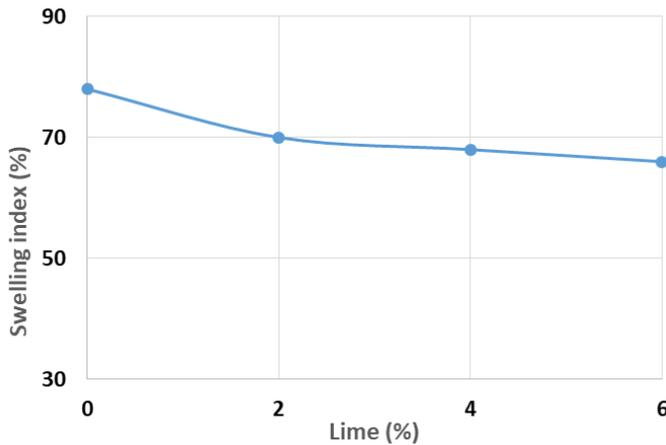
Figure 3. Influence of lime on free swelling index (the values are an average of the six soil samples)
