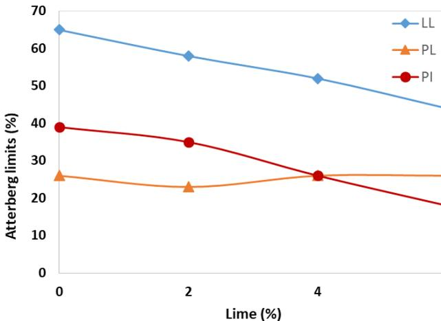
Figure 2. Influence of lime on atterberg limits (the values are an average of the six soil samples). LL = liquid limit, PL = plastic limit and PI = plasticity index
