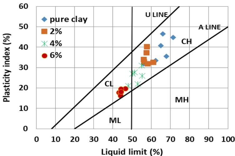
Figure 7. USCS classification of raw soil sample and after treatment with lime
